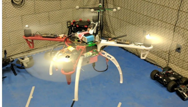
Figure 31: DJI Flamehwheel F450 with onboard Odroid-UX4 SBC and Optitrack ridged body markers positioned on the GPS Stand.
